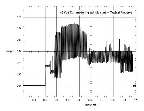
Figure 2. Typical 5V startup and operation current profile
